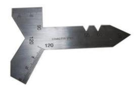
6.2 Total length: 95 mm ± 1 mm 6.3 Width: 45 mm ± 0.2 mm 6.4 Blade thickness: 1.5 mm ± 0.05 mm Blade material: 6.5 Stainless Steel 6.6 Should be handy and useful for grinding & setting thread cutting tools. 6.7 Satin chrome finish. Should have permanently deep etched graduations also edge profile ground. 6.8 6.9 Should be useful to find numbers of thread per inch by mean of given value. 6.10 Different angles are as per profile (rectangular, conical or edge cutting).
